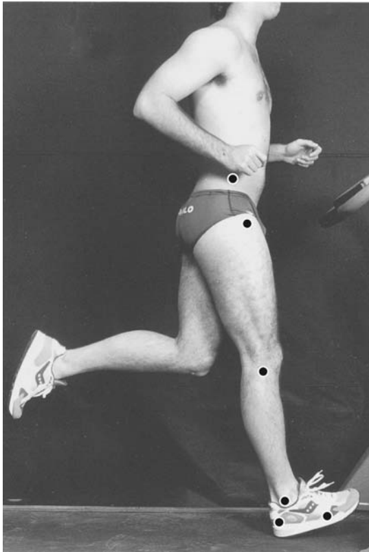
FIGURE 8-6 A runner marked for a sagittal kinematic analysis of the right leg.
