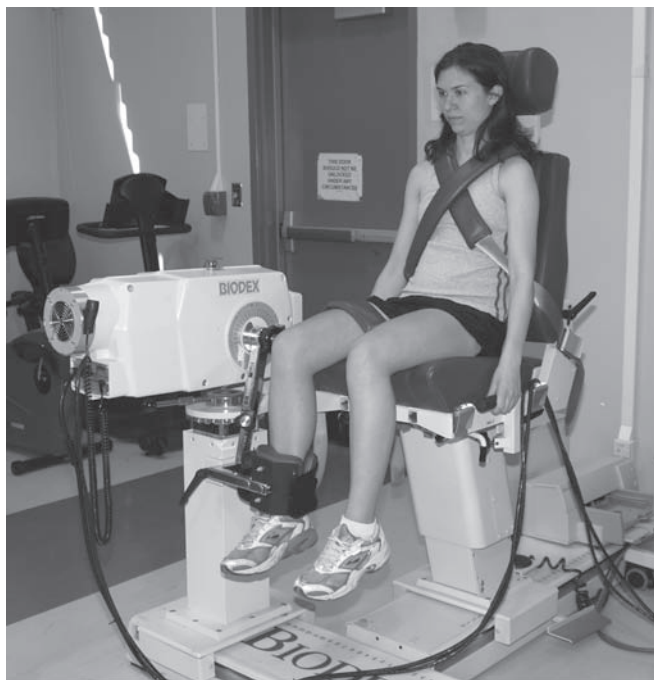
FIGURE 3-37 An isokinetic exercise for knee extension. The machine is the Biodes isokinetic dynamometer.
